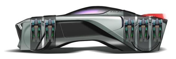
eLionJet is driven by 12 electrical ducted fan engines each with 1.000 N thrust; total 12.000 N.
